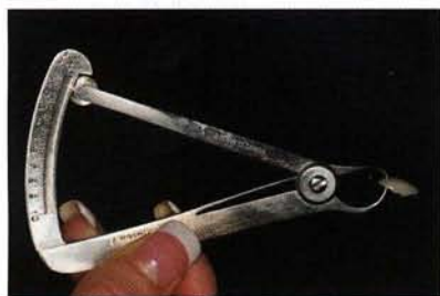
Figure 10 Micrometer measuring the thickness of the veneer.
