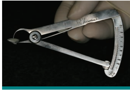
Figure 16 Boley gauge showing the thickness of the restoration to be 0.65 mm.
